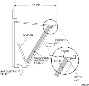
Fig. 3 - Filter Installation
